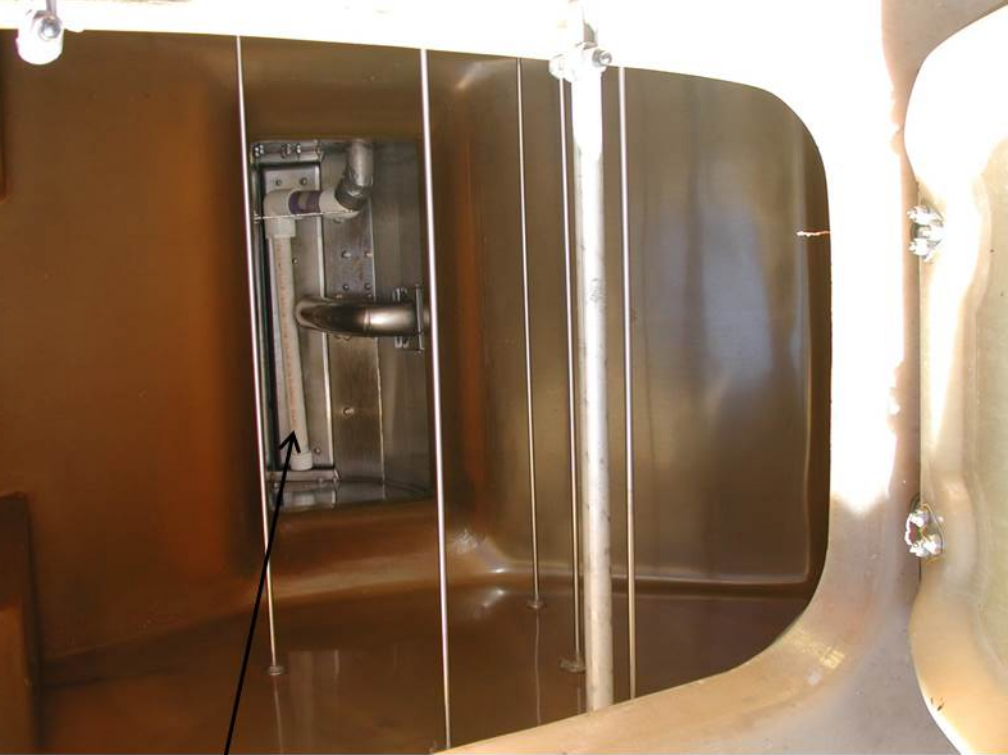
Example of air tube mounted in base of hopper
